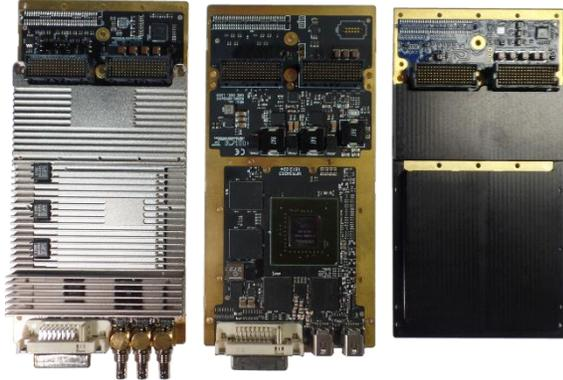
This module automatically detects and supports VPWR of +5V or +12V, comes with configurable power control options, and is configurable for ANSI VITA 42 (XMC 1.0) or ANSI VITA 61 (XMC 2.0).
