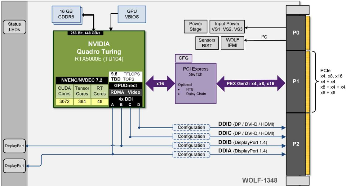
Standard model with video output over P2 or front panel connectors.
