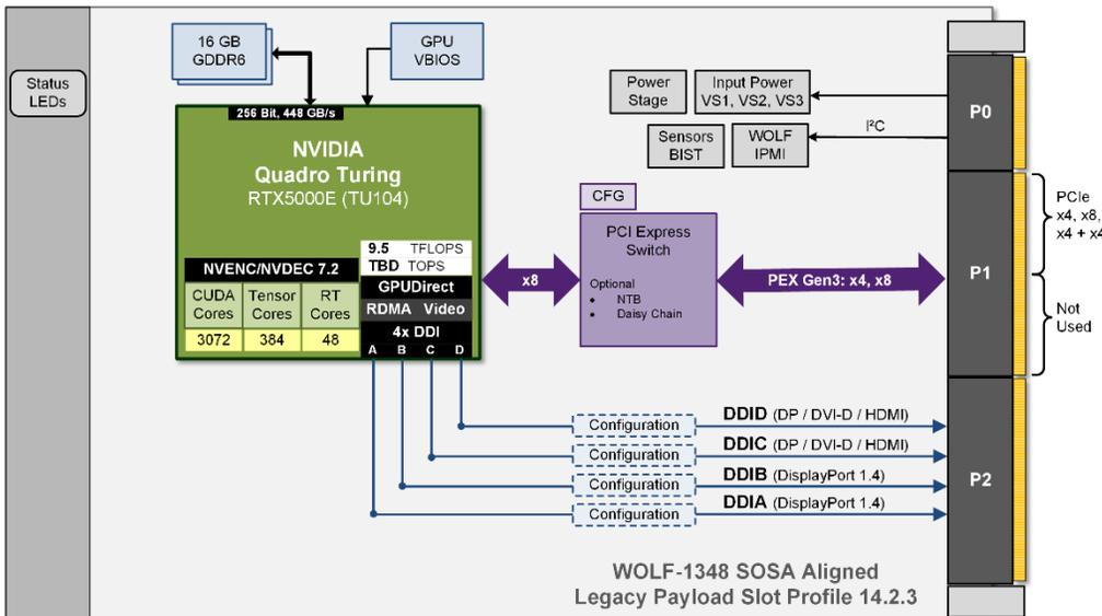
SOSA aligned model with support for Legacy Payload Slot Profile 14.2.3.
